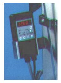
Note! H3i Controllers as supplied with H45 Kilns are supplied "Hard Wired" to the kiln and therefore do not have a Harting plug.
